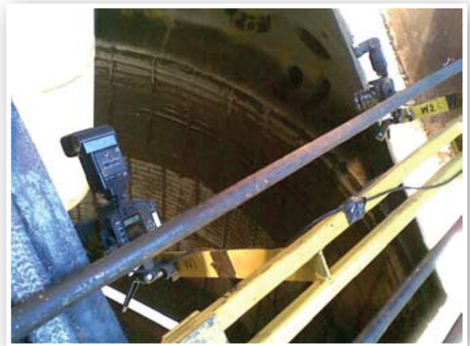
Above: Surface deformation analysis of the interior of a material bin and impact bars using specialised metrology software and dense 3D point cloud data.
