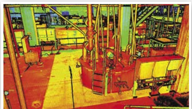
Screen capture of laser scanning of the process area at the platinum refinery
