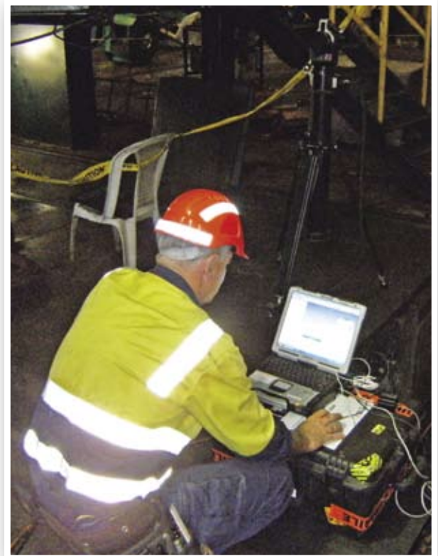
Above: Surveyor controlling the laser tracker
