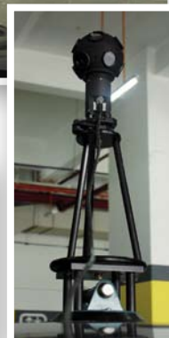
Figure 3: The SiteSeeV camera system mounted on the car capture platform
