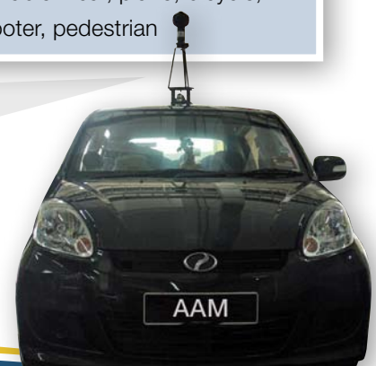
Figure 3: The SiteSeeV camera system mounted on the car capture platform
