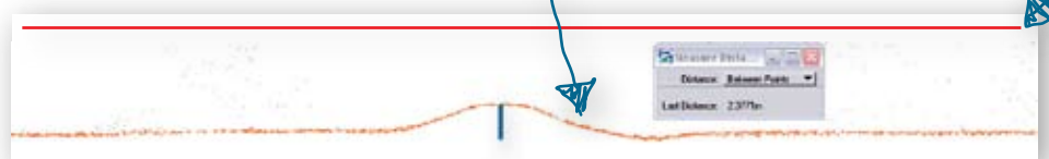
Below: The blue line shows the height of the levee at this location. In the image the orange points represent the original "all points" of ground data.
