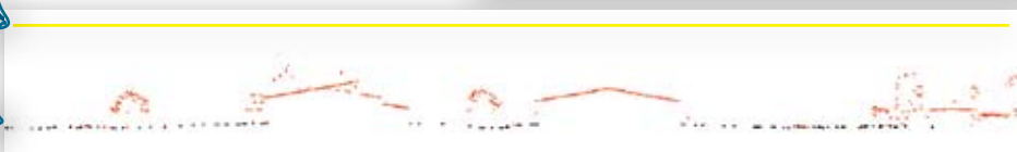
Below: Cross section – The orange (non ground) and black (ground) points provide a ground view of the yellow cross section shown in the above image.
